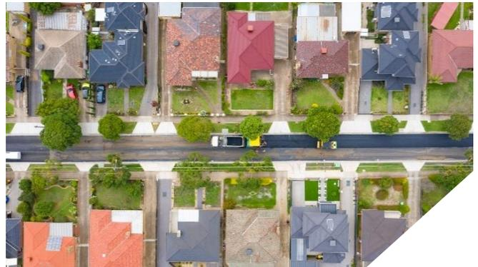
In preparation for the Department's trial, a first demonstration of the SMA10 material with OLEXOCRUMB<sup>®</sup> A20E was placed on a suburban street in Melbourne in March 2020. The 2400m<sup>2</sup> of SMA10 was laid successfully.
